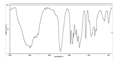
d) This is probably an ESTER – it has a carbonyl C=O @ 1700 and there is also a C-O peak @1000-1100 and @ 1300. (There could be a double Br peak down around 500-600, but it is more likely to be an ester. This could be confirmed using other spectra)
